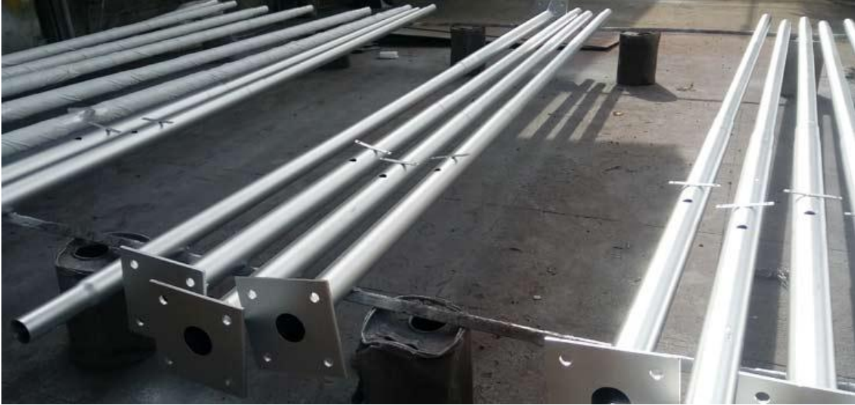
Fig l: 9meter long 410-SP-30 swaged steel tubular pole with CI base plate and cap
