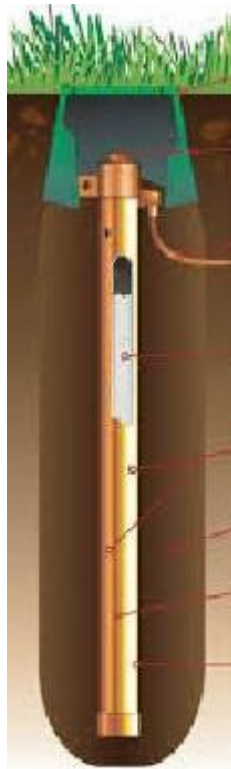
Fig j: safe earthing model T-19 of size 50 mm diameter * 2meter electrode
